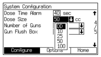
Fig. 26. Configure Screen 4, dynamic dosing selected
